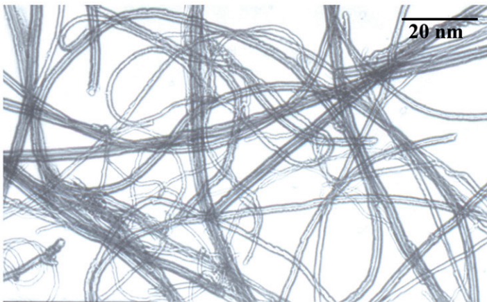
Figure 7. The TEM image of CNTs after purification stage from a bigger area.
